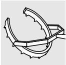
G-33757 CLEAR-CORNEA-INCISION FIXATION RING inside diameter 16.0 mm swivelable, 12 teeth
