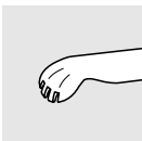
G-37575 MEMBRANE SPATULA 0.5 mm curved, short rakes, round edges 20 gauge / 0.9 mm
