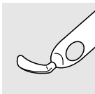
G-32055 THOMAS NEUHANN/SAUDER IRRIGATION HANDPIECE WITH CHOPPER irrigation ports 2 x 0.75 mm tube 19 gauge / 1.1 mm
